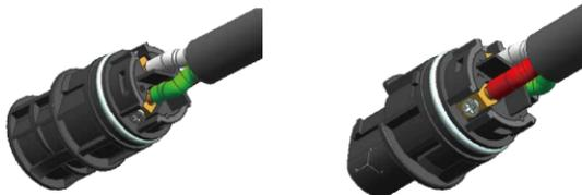
Push the male or female cable body into housing body correctly according to the position of the clamping groove, and will hear a crisp “click” sound in place.
